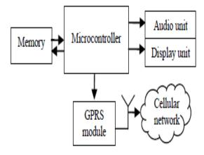
Fig.2 Station Unit Block Diagram
