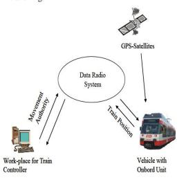
Fig.1 Schematic overview of automated system
